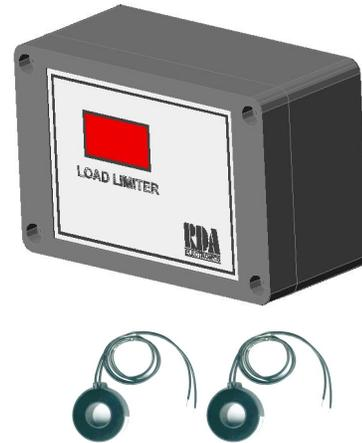
Times and currents are set digitally and stored in memory, the setting is simplified and requires no measuring instruments. Motor current is displayed on the screen during operation. Installation is simplified as each unit is supplied with a pre-wired cable and two current transformers (CT's).
